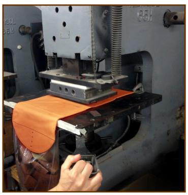
Once the piece is fully assembled, the section which will be on the spine of the book is foil stamped.
