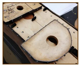
The first step is making the die which is used to cut the leather in the shape of the wrap.
