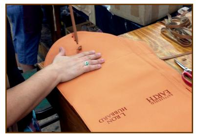
At the next station, the leather thong is threaded through the holes in the cover flap section.
