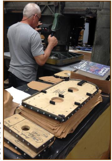
The die is then mounted on a press to cut the leather in the desired shape. The material used for the wrap is a soft, supple, genuine full-grain imported leather.
